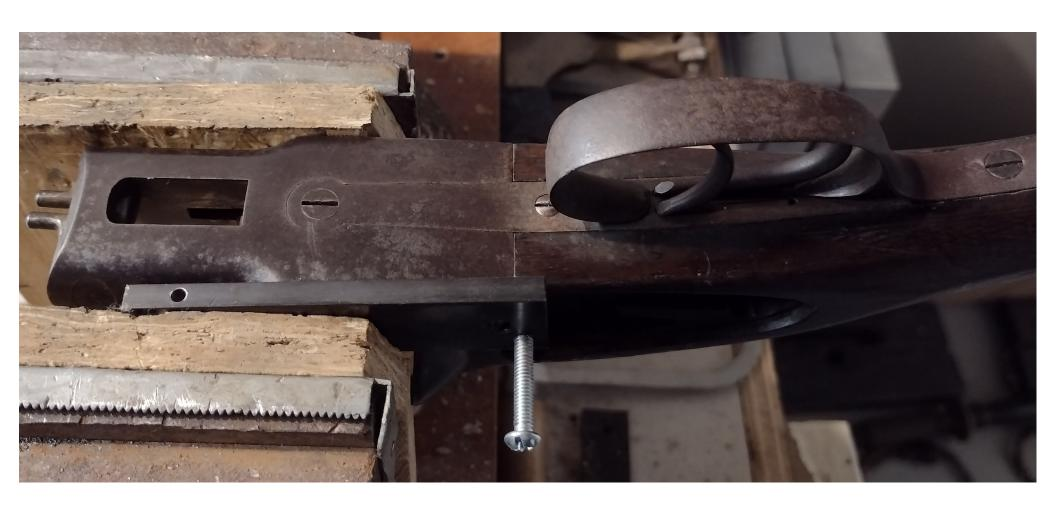
The arrow shows where the screw went, just behind the receiver. The gap between the stock and the receiver was barely the diameter or a #8 screw.
